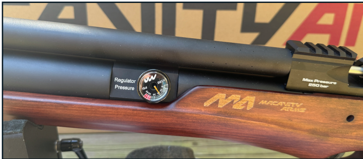
The regulator is externally adjustable to as low as 600 PSI to increase shot count.
